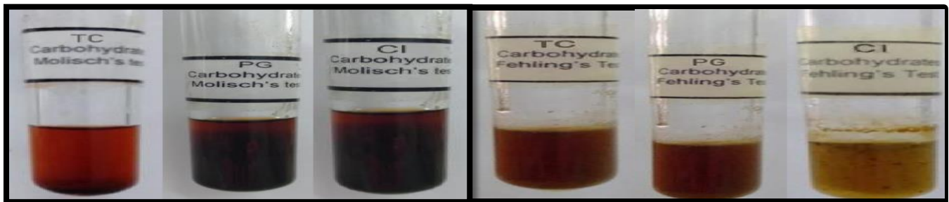
Figure 3: Phytochemical screening for carbohydrates (a) Molisch's test (b) Fehling's test
