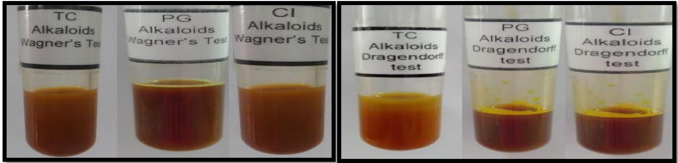
Figure 1: Phytochemical screening for alkaloids (a) Wagner's test (b) Dragendorff's test.
